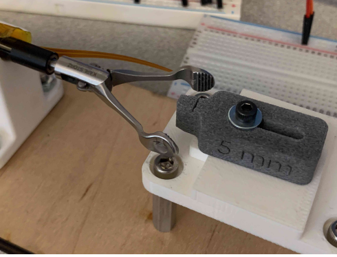
Fig. 7: Position calibration subassembly with 5 mm block.
